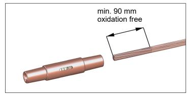
3. Insert the cable carefully into the cone. The cable end must be visible through the window.
