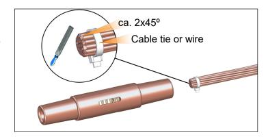
2. The cable should not be oxidized in the clamping part of the conical coupler. Oxidized cables should be cleaned with a wire brush.
